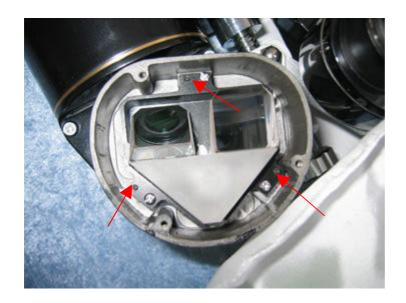
There are three screws on each prism cover plates, please loosen these three screws, then you can take off the cover plates from binoculars, and you can see the prisms as above picture, and there are three small focusing screws, you can use screw driver to adjust these focusing screws for collimation, and usually, our collimation standard for this binoculars on our collimation machine is:
