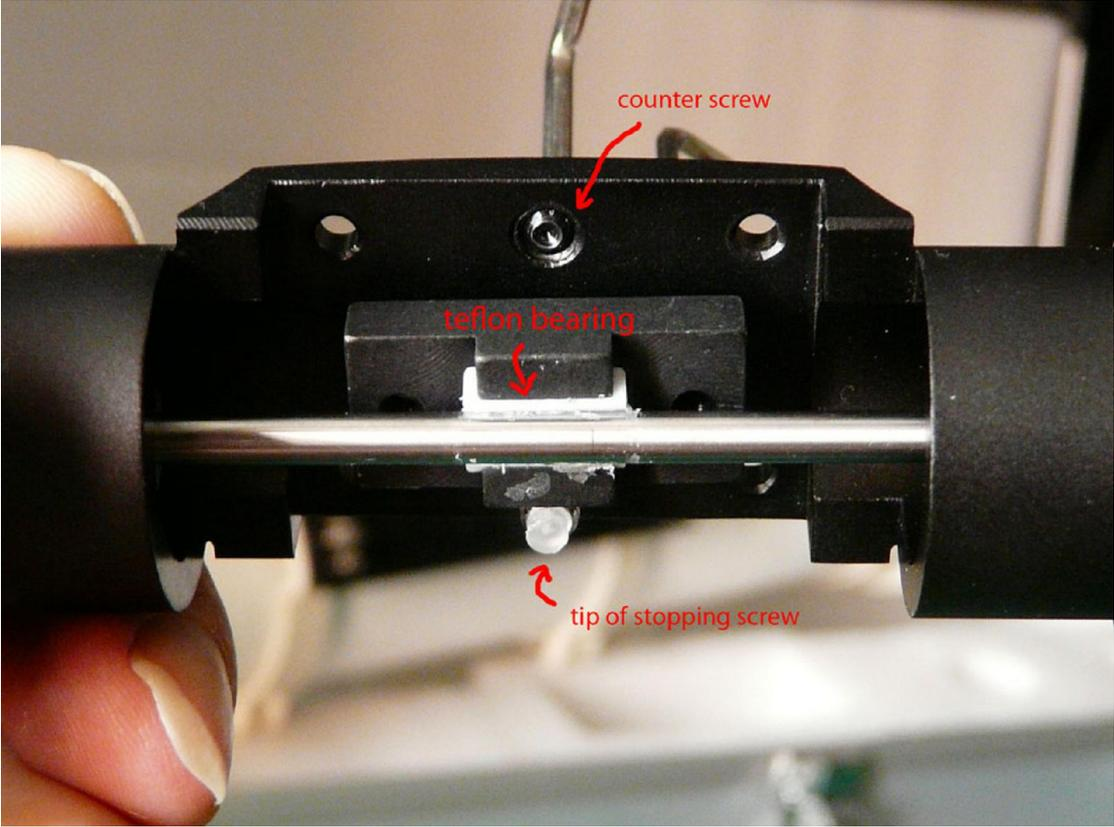
The holder of the teflon bearing can be tilted or parallelized to the shaft by the 2 screws left and right of the grip adjusting screw. At the same time they act as limiter for the pressure. If they are too tight, the focuser tube may slip, no matter how much you tighten the grip adjusting screw:
