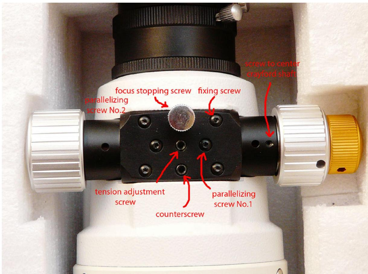
Here the 4 fixing screws have been removed – take care to keep that rubber rings at the threads of the fixing screws, they make for the final soft touch of the crayford:
