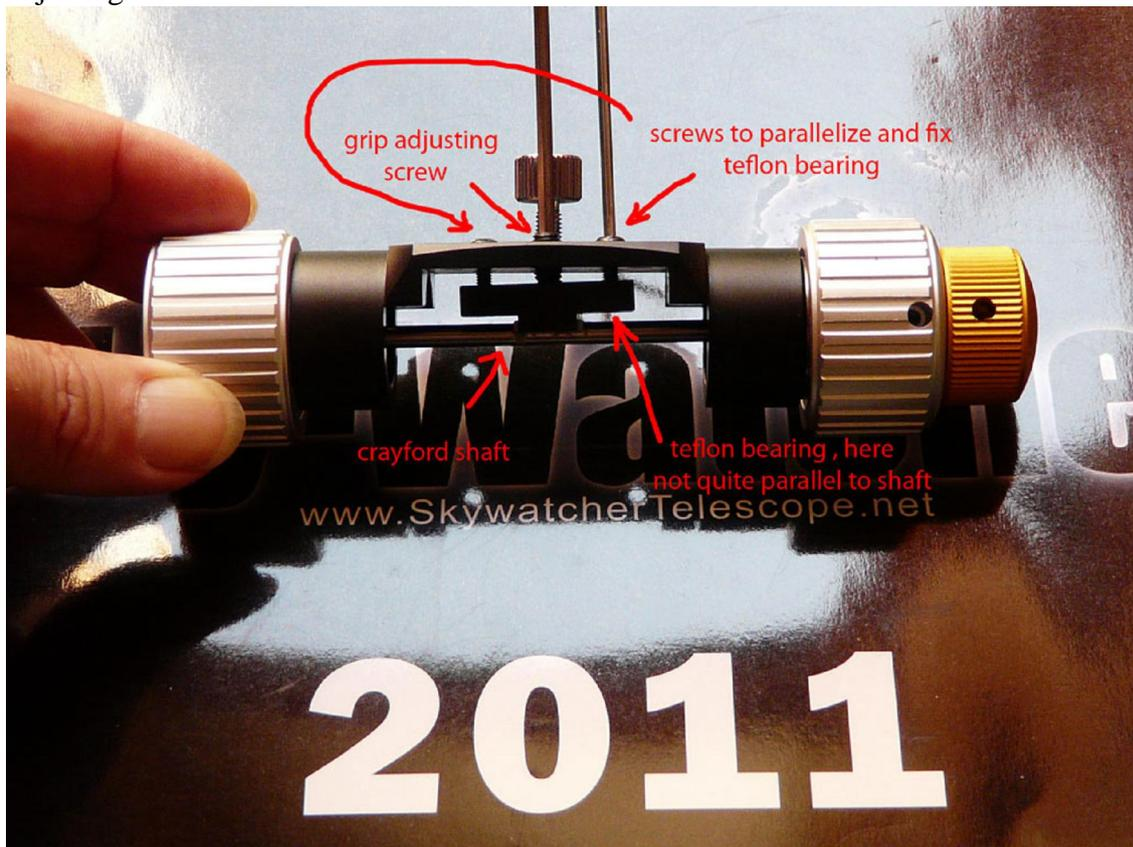
As you see, there are 2 systems counteracting – first the tension adjustment screw and the 2 screws nearby, second the counterscrew and the 4 fixing screws buffered by the rubber rings. It is a good idea to use the first system to make the course adjustment, and a little extra strength, and the second system to fine-tune that.
