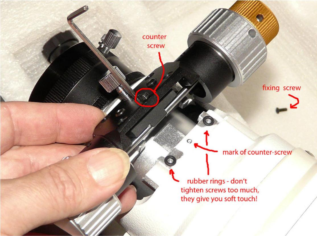
Here you see the teflon bearing where the crayford shaft is moving and the pressure for the right grip is applied:
