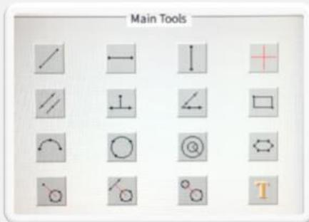
In the simple user interface, you can choose from 14 different measurement functions. Measurement data, text field and cross-linkable data can be attached to the image. The edge search function makes the measurements more accurate.
