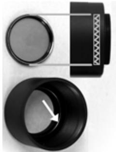
A 48mm (2") filter can be mounted inside the DSLR extender tube if needed. By example using a light pollution reducer filter may allow pictures of the night sky even in suburban areas.
