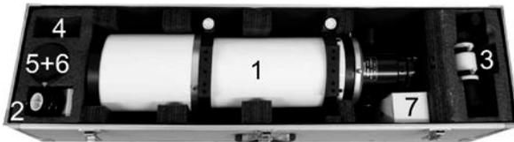
1. The telescope with dew cap retracted.
