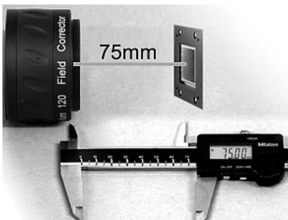
The 75mm distance is measured from the edge marking the start of the male thread on the field flattener, to the CCD sensor (see picture on the left).
