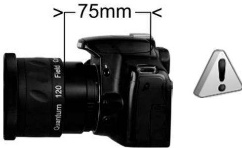
In order to get the premium results the field flattener for ESPRIT 120 can deliver the distance between the last lenses to the sensor should be exactly 75mm. This distance is called the field flattener "back focus".
