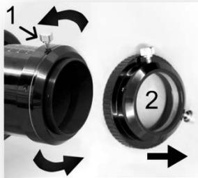
Before installing the field flattener onto the drawtube of the Helinear focuser, the 2" ring adaptor (2) needs to be unscrewed and removed.
