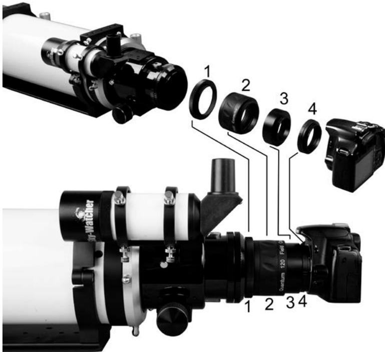
1. Screw the drawtube adaptor (1) at the end of the focus tube.
