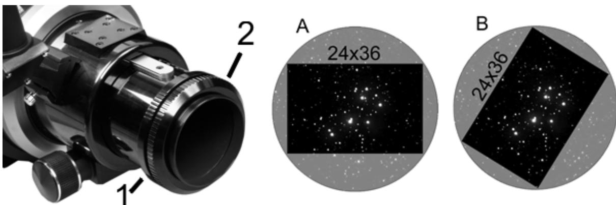
When the object you want to picture is in the middle of the circular 44mm field, most often its orientation on the rectangular camera sensor is not what you expected (figure A). You can easily reframe the picture on the camera sensor by unscrewing the blocking ring (1) at the end of the focuser drawtube, then turning the adapter ring (2) with all the optical train until the framing suits your needs (figure B). When done screw the ring (1) to lock position, and you are ready to picture the sky.
