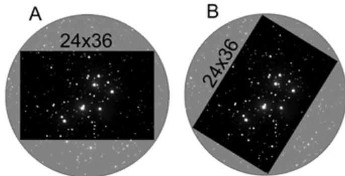
When the object you want to picture is in the middle of the circular 44mm field, most often its orientation on the rectangular camera sensor is not what you expected (figure A). You can easily reframe the picture on the camera sensor by unlocking the thumbscrew at the end of the focuser drawtube and turning all the optical train until the framing suits your needs (figure B). When done relock the thumbscrew, and you are ready to picture the sky.
