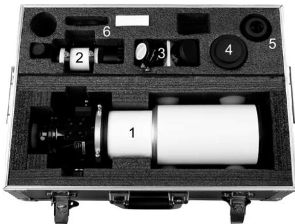
1. The telescope with dew cap and EQ5 (Vixen style) dovetail bar.
