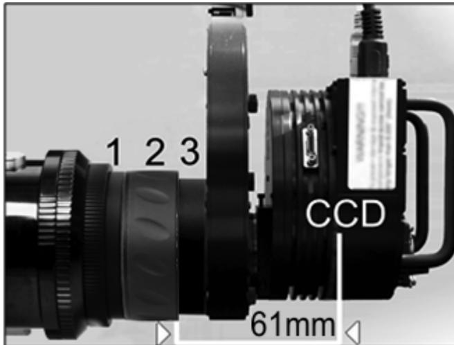
1. Screw the drawtube adaptor (1) at the end of the focus tube.
