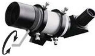
If it is necessary to refocus your finder scope, sight on an object that is at least 500 meters (or yards) away. Loosen the locking ring by unscrewing it back towards the bracket. The front lens holder can now be turned in and out to focus. When focus is reached, lock it in position with the locking ring.
