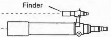
A finder is a useful tool. It permits the precise centering of an object in the field of view. The 6.3-degree field of view allows the easy centering of an object to be viewed or photographed.
