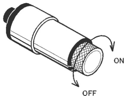
In order to turn the illuminator on, turn the knob clockwise. The knob will click when the illuminator turns on. As the knob is turned, the reticle will brighten. Adjust the knob to the desired brightness. Turn the knob counter-clockwise past the click to turn the illuminator off.
