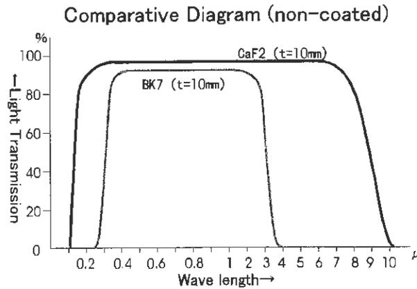
As the diagram shows, the band pass of fluorite of 1000 to over 100,000 angstroms eclipses by many magnitudes that of any optical glass. Additionally, the use of multicoatings further increases light transmission over any ED glass. These features make the fluorite objective the premier photo/visual instruments for deep sky or lunar and planetary applications in their size class.
