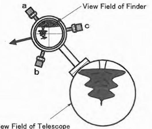
2. In order to move the crosshair in the direction of the arrow, first loosen screw (a) and tighten (push) the finder with screw (c). This procedure will move the crosshair in the desired direction. The top of the finder will move in the opposite direction and the object will move in the direction of the smaller arrow.
