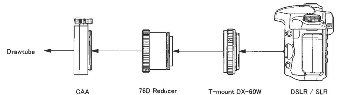
Connection for magnifying imaging with the Extender-Q 1.6X
