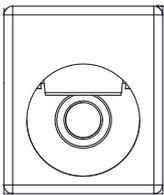
12 V DC power input for charging the internal battery and direct supply of power for operation of the FUSION-120i mount.
