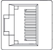
Hand controller port RJ-12 for optional SynScan hand controller.
