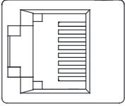
Autoguider port for use in equatorial mode during astrophotography.
