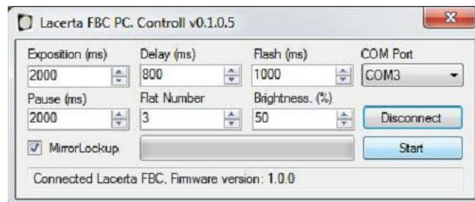
After connecting, the program checks the connected device. When connecting another device, the connection is interrupted. After connecting Lacerta FBC successfully, it shows the device firmware version number. If the Lacerta FBC is not connected in Serial mode, you will receive a warning:
