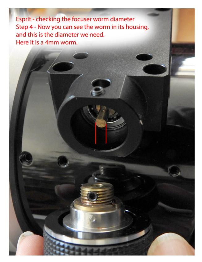
Please measure the diameter using a gauge and order your MFLA motofocus with the according coupler.
