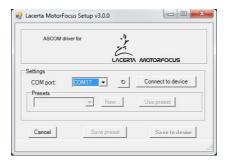
The serial port of **LACERTA MFOC** can be selected in the COM port drop-down menu. When the connection is created, parameters are loaded from Eeprom. After parameter modification click the "Save to device" button to write changes into the Controller. Depending on the controller's own characteristics, you can override the submitted value.
