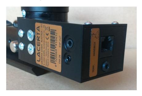
left side: 2,5mm stereo socket (from MGEN's camera port)
