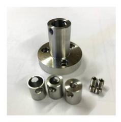
Slip the proper spacer Inlay into the 9,5mm cavity and align the holes with the threads in the coupler. Slip it over your worm, so the screws are able to contact the worm directrly. Using the proper length hex screws (2 pcs, 180° positions) fix the coupler to the worm, but at first not tightly. First, turn the focuser worm manually to allow the coupler aligning with the worm, when done only then fix the coupler to the worm tightly, and the motor to the worm housing.
