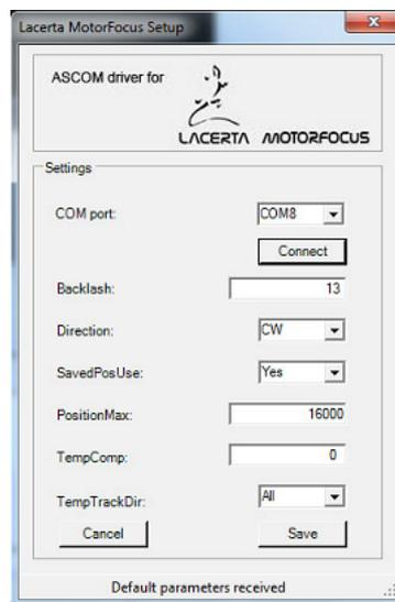
The serial port of **LACERTA MOTORFOCUS** can be selected in the COM port drop-down menu. When the connection is created, parameters are loading from Eeprom. After parameter modification click the Save button to write changes into Controller.
