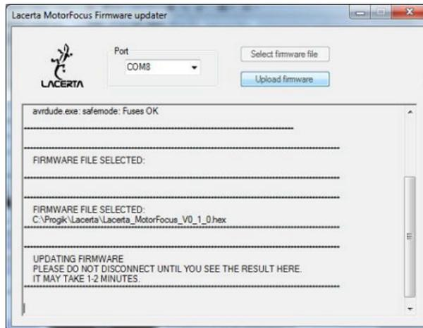
To start uploading, press the **Upload firmware** button. An uploading message at the bottom of the window shows the process status. When the uploading is in progress, the display of the Hand Controller is dark and the LED light of the serial communication is flashing. Red flashing is the sign of back reading.
