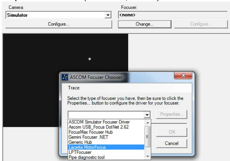
If the port was chosen previously, the device can be connected by pressing the OK button. A acoustic signal and flashing of device display indicate that the connection is created. „A” character shows in the **MOTORFOCUS** display that the **ASCOM** connection is available. For device parameters press the properties button.
