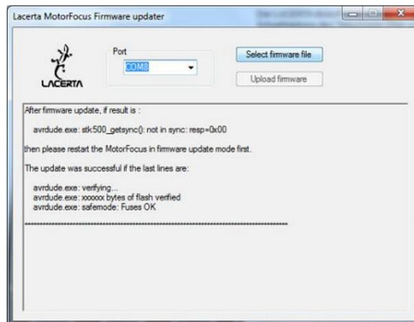
Select the port which is in use by the device (consult Device Manager if you don't know). Load the new firmware file with **Select firmware button**.
