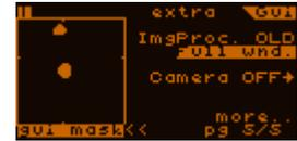
Now we press SET on the "Full wnd." item. A "choose point" text appears here and a little cross in the guiding window. Using the direction buttons we select a starting point for the partial method: we show the device which star we want to use for guiding, by pressing SET. From now the star is chosen and the guiding frames will be processed only 'partially', starting from the previous positions.
