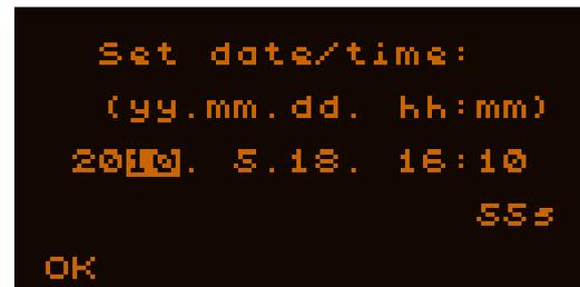
This screen appears right after power-on (from Firmware 01.21). If the filesystem is to be used set the date and time properly, timestamps will be inserted into the file.
