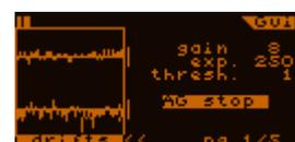
This is a time diagram (or history) of the drifts of the guiding star, relative to the guiding center where the star should be held. The latest 48 drift values are shown for the latest 48 frames, for each axis. One time step (one frame) is one pixel horizontally while vertically the drift values are scaled to the tolerance limit set. The tolerance interval is shown right next to the frame with two short lines, the size of it is  $\pm 4$  pixels to the zero.
