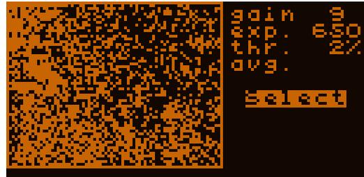
Each displayed pixel corresponds to a 10x10 pixel field on the CCD surface, its 'brightness' is derived from those. The method of calculation the brightness is described later.
