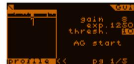
The horizontal line in the window (inverted pixels) shows the actual threshold value for each frame.
