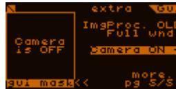
(If You don't see the star again after 'Camera ON', the guiding optics or mount must be moved or rotated.)
