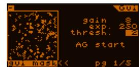
This page contains the parameters of imaging and the autoguiding can be started and stopped from here.
