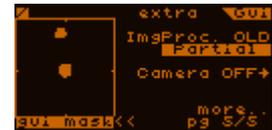
If the NEW image processing method is selected, you can only set a new point for the algorithm and "Partial" is always shown, because the NEW method involves the partial feature.
