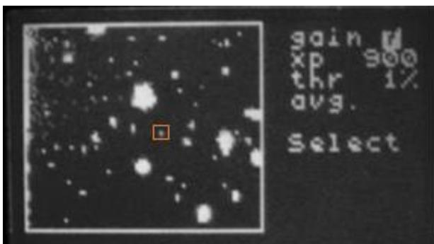
Using the live view, focus until stars appear smallest. Now mark "select" and press SET. A small rectangle appears on the screen, and you can use the directional buttons to move it and place it onto a star.
