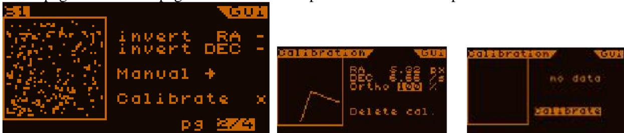
On the Calibration screen mark "Delete cal." if there has already been a calibration before, or press directly "Calibrate". Watch the calibration routine taking place, moving DEC, moving RA and finally finishing and outputting some values. Orthogonality is good over 90%. The mount is driven to the start position before calibrating, and by pressing ESC twice you return to the guiding window.
