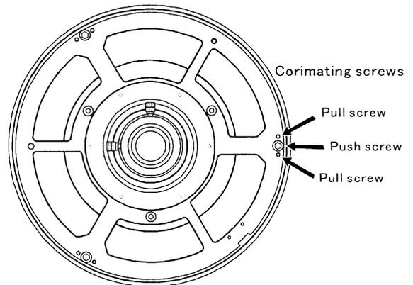
The collimation for the primary axis is made with 3 sets of the pull screws and 6 sets of the push screws, by using Allen wrenches provided. Refer to the Fig. 20.
