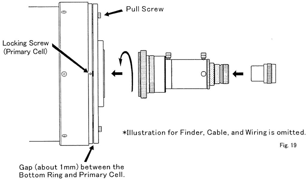
In case the inner and outer image of a star does not become a concentric circle after the secondary has been collimated, collimation for the primary can be done with the following procedure.
