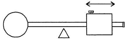
The next step is to place the tube assembly parallel to the ground with the counterweight shaft parallel. Holding the counterweight shaft with one hand, loosen the RA clamp. Let go of the counterweight shaft and see if the assembly moves. If the scope is not balanced, carefully slide the counterweights to a point where the telescope is balanced.
