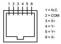
shows the Pulsar2 autoguider socket pinout. STV needs a reversed cable, STAR2000 a direct cable.
