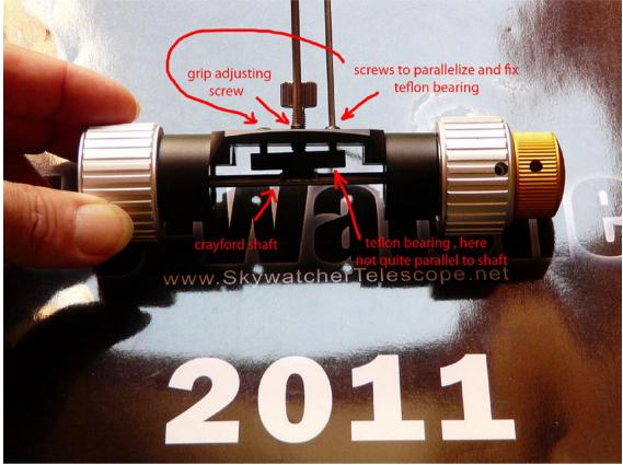
As you see, there are 2 systems counteracting – first the tension adjustment screw and the 2 screws nearby, second the countersrew and the 4 fixing screws buffered by the rubber rings. It is a good idea to use the first system to make the course adjustment, and a little extra strength, and the second system to fine-tune that.
