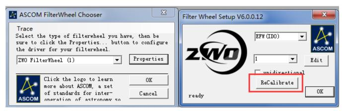
3. I use 7-position EFW, normally I had slots 1, 2, 3, 4 filled and slots 5, 6, 7 empty, but then I got the error below and the EFW stopped working. I checked the carousel. It was not too tight or loose.
