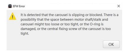
When using the filter wheel it is very important to keep its internal balance. The weight and distribution of the filters will affect balance. Thus we recommend you space the filters out and evenly distribute them. In this case, install them in slots 1, 3, 5 and 7, then the EFW will work again.
