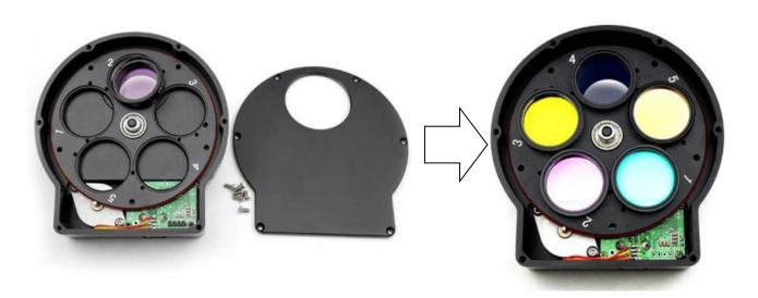
For 31mm, 36mm & 51mm unmounted filters: (Please use the M2 screws and washers to fix the filters, which are included in the package.)
