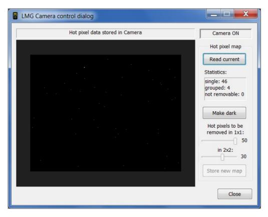
"Statistics" gives some info about the amount of different hot pixel types. Single hot pixels are surrounded with normal (non-hot) pixels. A grouped hot pixel is such that it has at least one neighbouring hot pixel. These could be cosmetized as well but with less efficiency, since there are less surrounding good pixel information. Not removable hot pixels are totally surrounded by another hots, these are very rare and won't be cosmetized at taking frames.
