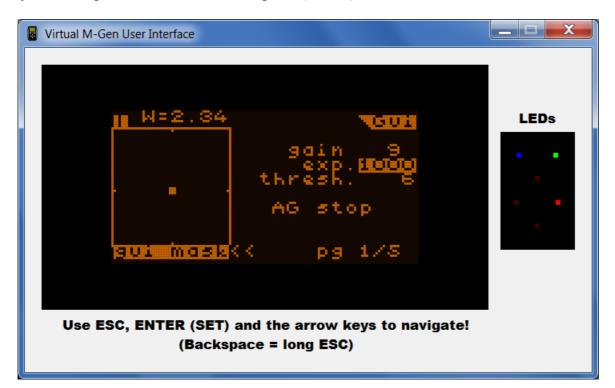
The display here is exactly the same as on the HC's LCD display. The buttons are replaced by the PC's keyboard with the following mapping:
