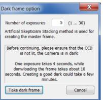
Ensure that the CCD is not lit even a little bit. The exposures are 4 seconds long and taken at high gain (sensitivity).
