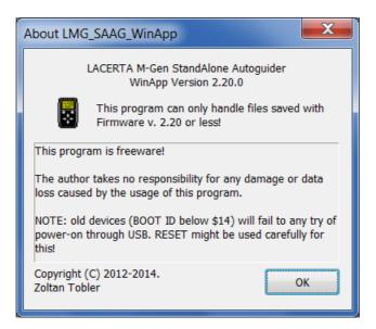
The PC application's version show that highest verison number of the Firmware in the device that it can handle. There is always a new PC application for each new Firmware release. The users are advised to use the PC app. version equal to the running firmware to avoid some incompatible behaviour.
